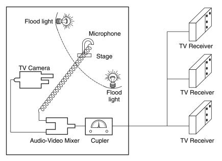
Fig. Simple closed circuit TV system
